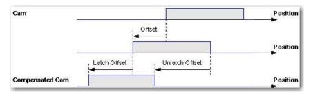
The cam range is defined by the left and right cam positions of the Output Cam element. The compensated cam range is defined by the cam range, offset, and latch and unlatch offsets. The latch and unlatch offsets are defined by the current speed v.
