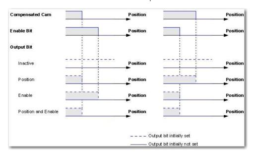
The following diagram shows the effect of the selected unlatch type on the output bit for different compensated cam and enable bit combinations as function of time.
