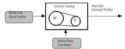
Actual position is the current position of a physical axis as measured by the axis encoder. This is the only valid selection when the master axis' Axis Type is configured as Feedback Only.
