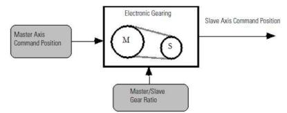
Command position (only valid when the master axis' Axis Type is configured as Servo) is the current desired or commanded position for the master axis.
