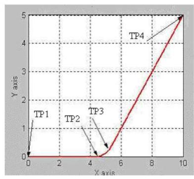
The following table shows the bit status at the various transition points shown in the preceding graph with termination type of Command Tolerance. For Command Tolerance termination type distance-to-go for transition point TP2 is equal to Command Tolerance for the Coordinate System cs1.
