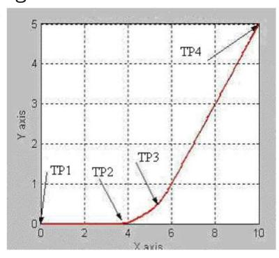
The following table shows the bit status at the various transition points shown in the preceding graph with termination type of No Decel. For No Decel termination type distance-to-go for transition point TP2 is equal to deceleration distance for the Move1 instruction. If Move 1 and Move 2 are collinear, then Move1.PC will be true at TP3 (the programmed end-point of first move).
