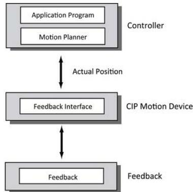
No Control mode also applies to other CIP Motion device types, such as standalone Bus Power Converters and dedicated Motion I/O device types. Since there is no feedback channel that is associated with these device types, no actual position is returned to the controller.
