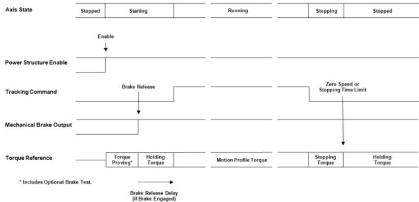
**Tip:** Recommended criteria for Zero Speed is based on Velocity Feedback, or in the case of Frequency Control drive, based on Velocity Reference. Zero Speed criteria can be established explicitly through optional Zero Speed and Zero Speed Time attributes or implicitly as 1% of motor rated speed or left to the drive vendor's discretion.
