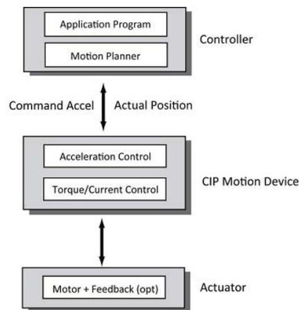
A feedback device for the acceleration control configuration is mandatory and may be used to return actual position, velocity, and acceleration data to the controller using the cyclic data connection.
