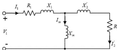
For permanent magnet motors, the Motion Control Axis assumes all motor parameters are defined in the context of a phase-to-phase motor model.
