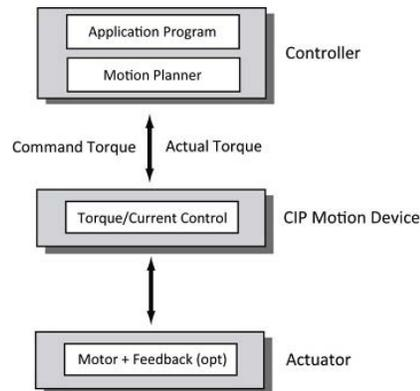
A position feedback device for this control mode is optional. If a feedback device is present it can be used to return actual position, velocity, and acceleration data to the controller using the cyclic data connection.
