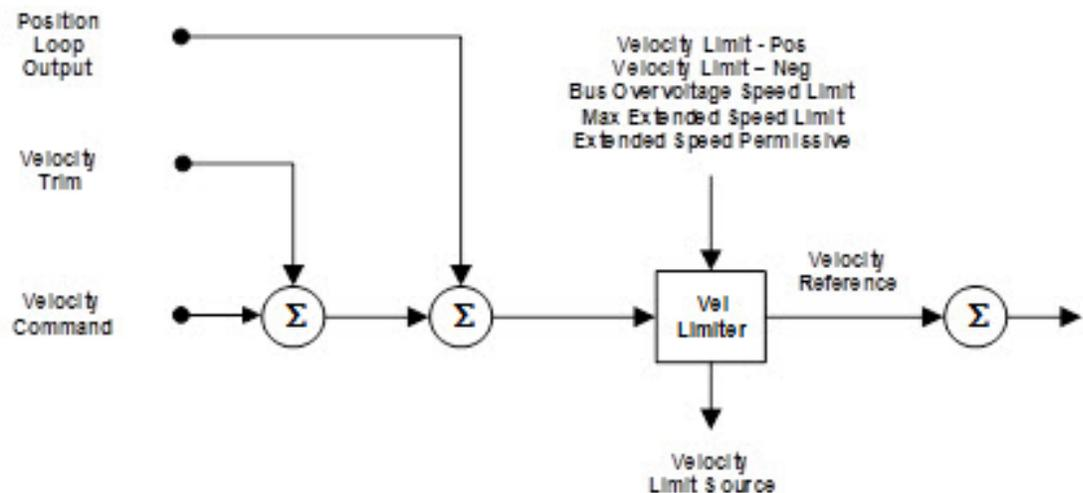
Through these extensions to the Velocity Limiter function, a drive that supports field weakening can be configured to safely manage extended speed operation, only allowing operation above  $S_{OV}$  by setting the PM Motor Extended Speed Permissive attribute. Systems that can run safely above  $S_{OV}$  are generally equipped with a DC Bus Regulator or a Resistive Brake Module.
