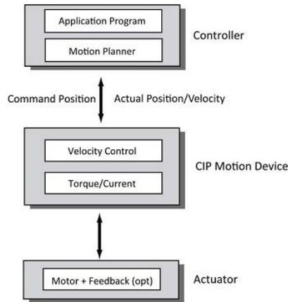
A feedback device for the velocity loop drive configuration is optional. You can achieve tighter speed regulation when using a feedback device, particularly at low speed. When the feedback device is included it may be used to return actual position, velocity, and acceleration data to the controller using the cyclic data connection. When the feedback device is not included, only estimated velocity can typically be returned to the controller.
