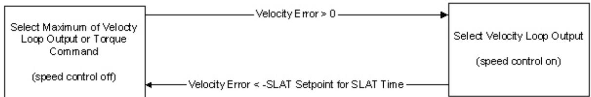
The active 'Max' select function will select the larger, or Max function, of the Velocity Loop Output or the Torque Command. The Velocity Command value is a negative quantity and so when the motor speed is mechanically limited, the Velocity Error is a negative value, and the Velocity Loop Output is a saturated (limited) to a negative value. The Torque Command is also negative, but smaller in magnitude, so it becomes selected by the 'Max' operation.
