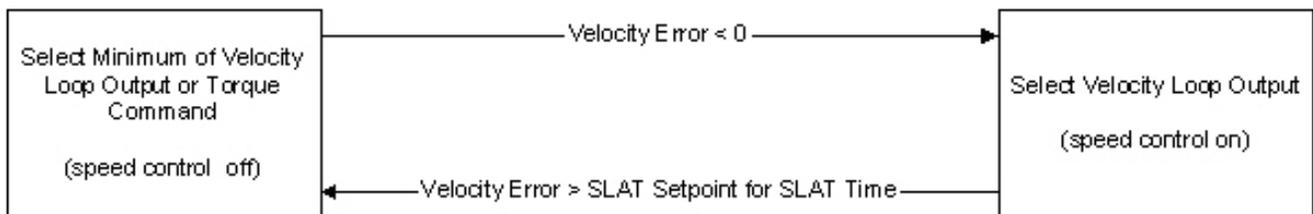
When used for SLAT control, an application dependent Velocity Command is applied to the drive. When the motor's speed is mechanically limited, this reference is at a level that results in saturation of the velocity loop output. In this state, the 'Min' select operation selects the smaller Torque Command value. The Velocity Error is positive in value equal to the Velocity Command.
