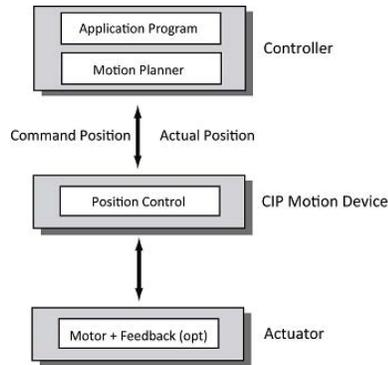
A feedback device for this configuration is optional. In the absence of a feedback device, actual position can be estimated by the drive and returned to the controller.
