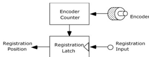
The Registration Latch mechanism is controlled two Event Control instructions, MAR (Motion Arm Registration) and MDR (Motion Disarm Registration).
