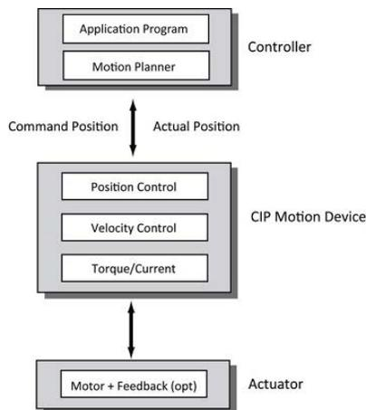
A feedback device for this configuration is generally required to achieve good positioning accuracy. The feedback device can also be used to return Actual Velocity and Actual Acceleration data to the controller using the cyclic data connection.
