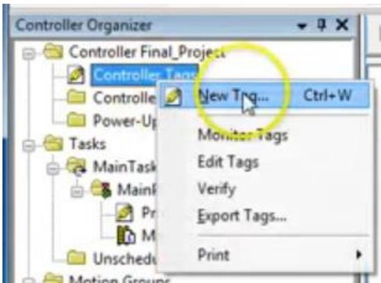
We will create a tag called "Signal\_to\_be\_sent", it is a **Produced** type tag, this will cause the data type to become DINT. Now click the **Connection** button and confirm the entry for Max Consumers is set to 1.
