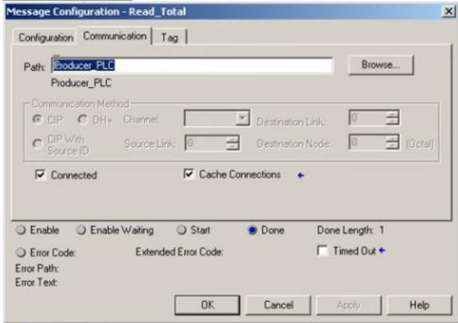
**Path:** brings up the network tree so you can select the other hardware. In this case we are selecting the **Producer PLC**.
