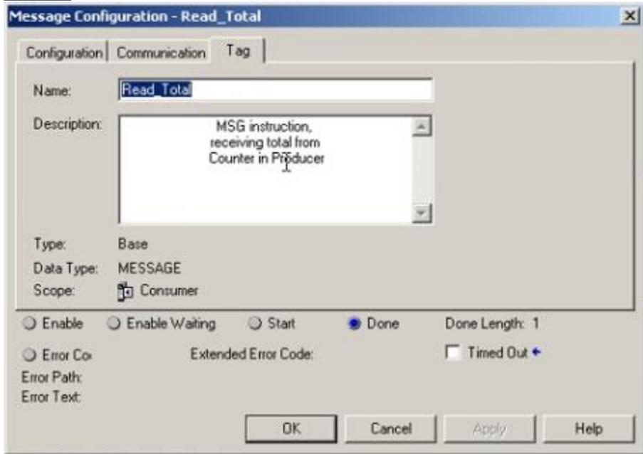
**Name:** the name given to the IO block. This is not the data tag!
