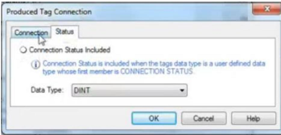
Now we create a simple program with the contact being a local input and the coil being on the other plc. But first we must specify which bit inside the data type DINT we wish to send. We can only send 1 bit.
