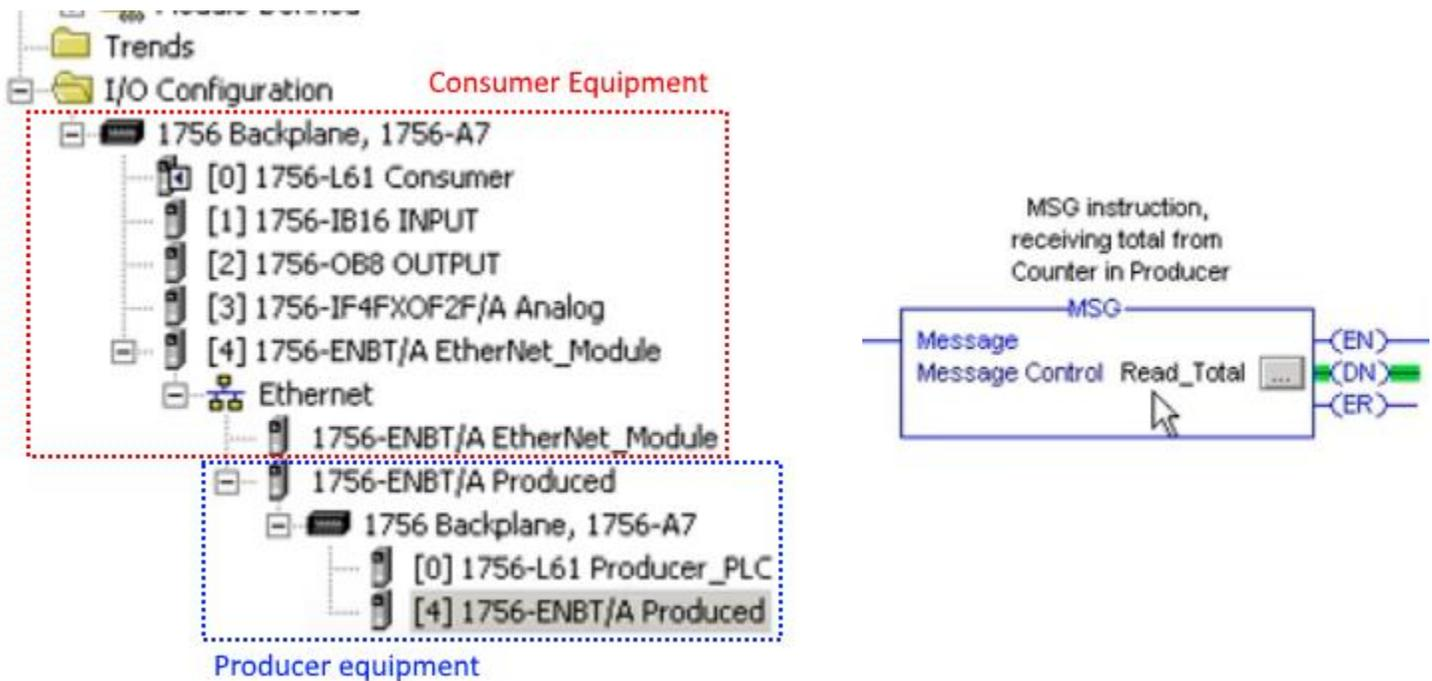
Message instructions must have a name, the example above is named Read\_Total. Keep in mind this name is not a tag, it, the name, does not transmit or receive data. Now click the eclipse to bring up the configuration dialog box.
