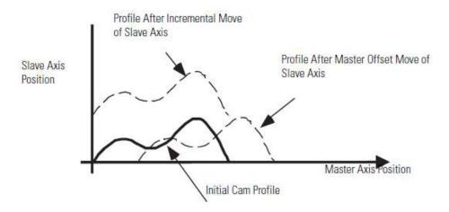
When the MAPC instruction (except pending) is initiated, the corresponding active Master Offset Move is disabled and the corresponding Master Offset, Strobe Offset, and Start Master Offset are reset to zero. In order to achieve the master reference position shift, the MAM instruction must be initiated after the MAPC is initiated.
