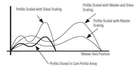
By default, both the Master Scaling and Slave Scaling parameters are set to 1. To scale a position cam profile, enter a Master Scaling or Slave Scaling value other than 1.
