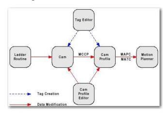
The data within the Cam Profile array can be modified at compile time using the Cam Profile Editor, or at run-time with the Motion Calculate Cam Profile (MCCP) instruction. In the case of run-time changes, a Cam array must be created in order to use the MCCP instruction.
