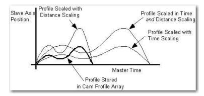
When a cam profile array is specified by an MATC instruction, the master coordinate values defined by the cam profile array take on the time units (seconds) and the slave values take on the units of the slave axis. By contrast, the Time and Distance Scaling parameters are unitless values that are simply used as multipliers to the cam profile.
