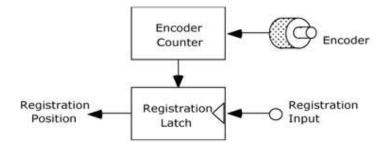
The Registration Latch mechanism is controlled two Event Control instructions, MAR (Motion Arm Registration) and MDR (Motion Disarm Registration).
