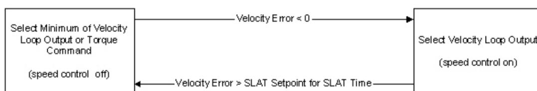
When used for SLAT control, an application dependent Velocity Command is applied to the drive. When the motor's speed is mechanically limited, this reference is at a level that results in saturation of the velocity loop output. In this state, the 'Min' select operation selects the smaller Torque Command value. The Velocity Error is positive in value equal to the Velocity Command.
