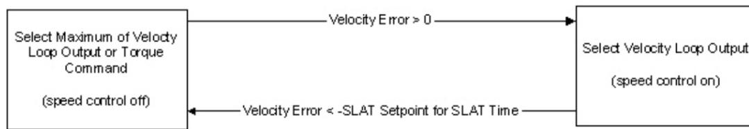
The active 'Max' select function will select the larger, or Max function, of the Velocity Loop Output or the Torque Command. The Velocity Command value is a negative quantity and so when the motor speed is mechanically limited, the Velocity Error is a negative value, and the Velocity Loop Output is a saturated (limited) to a negative value. The Torque Command is also negative, but smaller in magnitude, so it becomes selected by the 'Max' operation.
